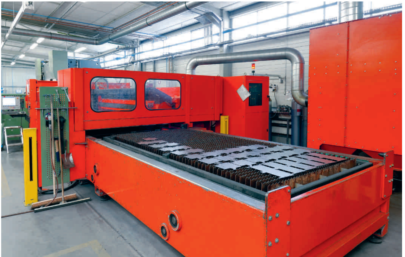
Durable: the 3,000-watt Bystar 3015, built in 2000, is fully integrated into production of parts.
