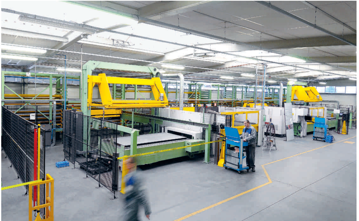
Part production at Mercedes-Benz Molsheim is dominated by small batch series and individual parts. Bystronic laser cutting systems and a fully automated Antil storage system provide the required flexibility and speed.
