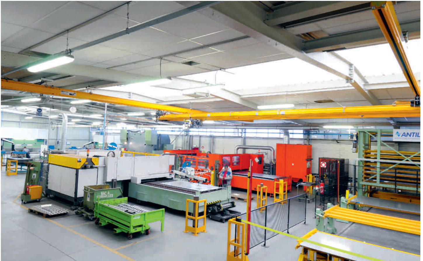
Customized truck conversion is a growing business sector for Mercedes-Benz that generates a significant need for laser parts. In total, the Molsheim factory operates four laser cutting systems, including these two Bystar stand-alone machines.
